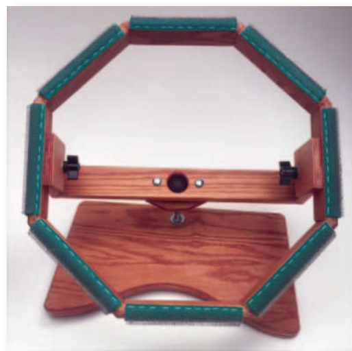
This frame is not labeled and the hooker does not know the brand. It looks very similar to a K’s Creation Octagonal Sit-on Frame. It tilts and turns on a ball joint. Adjustments are made by loosening and tightening the screws.
